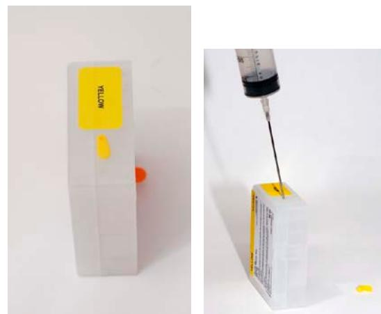
Always shake ink bottles before filling or refilling cartridges to ensure pigment is in suspension for consistent output.
